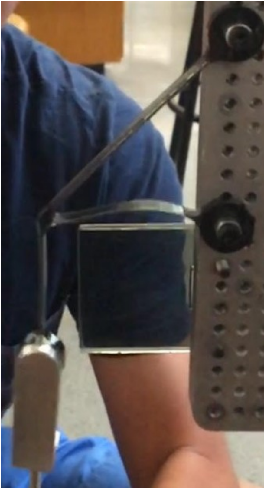
Screenshot of a slow motion video of an early design where we forgot to consider buckling. The part failed due to the compressive member being too thin to resist buckling.
